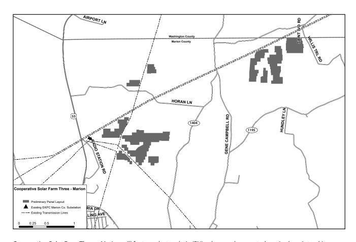
Cooperative Solar Farm Three - Marion will feature photovoltaic (PV) solar panels mounted on single-axis tracking systems supported by steel posts. When operating, the solar panels will move to track the sun from east to west over the course of the day. The solar farm will have capacity to generate 96 megawatts of electricity at alternating current (AC). That is enough to serve the annual electricity needs of 10,940 typical Kentucky homes.
